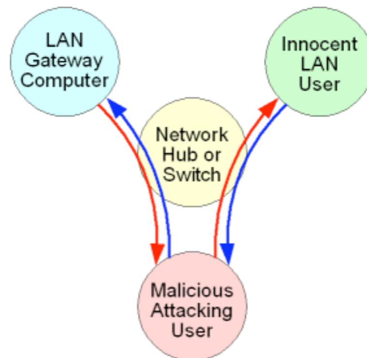
This "ARP Cache Poisoning" can be used to redirect traffic throughout the LAN, allowing any malicious computer to insert itself into the communications stream between any other computers for the purpose of monitoring and even alter the data flowing across the LAN.
